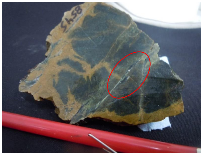
Figure 2: Piller 2012 - fine grained awaruite within ultramafic sample from the Atlantic Lake area, northern Pipestone Project area.
