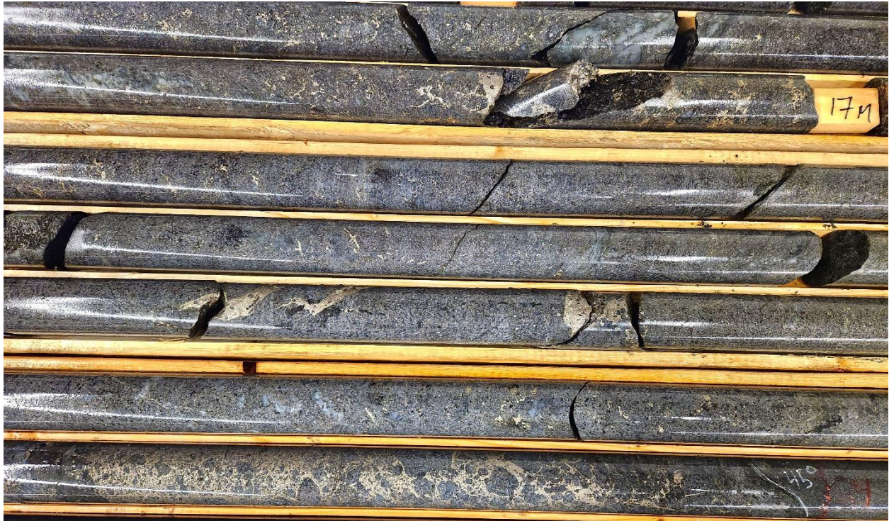
Figure 1: New drill core from VW-23-03 showing partial section from 15 metres to 24 metres. Interval of visual sulfides with pyrrhotite and visually identified interstitial chalcopyrite and pentlandite within the pyrrhotite showing disseminated to blotchy and net-texture. Bottom contact at 45 degrees.
