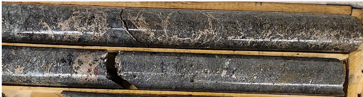
Figure 2: Drill hole VW-23-03 section from 1 to 4 metres downhole showing disseminated coarse patches of pyrrhotite with visually identified interspersed chalcopyrite and pentlandite within pyrrhotite.
