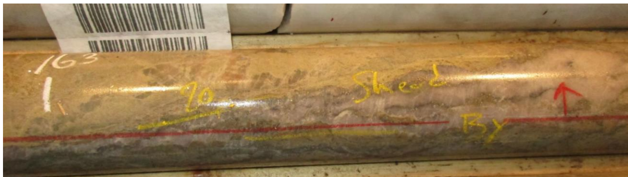
Figure 4: Hole 11 (ACP-R-21011) at 163.0 metres showing mineralized shear-parallel quartz carbonate vein with perpendicular extensional tension gashes/growth fabric.
