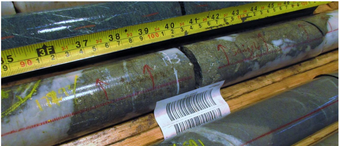
Figure 2: Hole 14 (ACP-R-210014) at 173.0 metres showing semi-massive sulphide intersection contained within newly intersected fourth quartz-carbonate veining zone.
